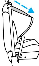
3. Allow the belt to retract. As the belt retracts, you will hear a clicking sound. This indicates the safety belt is now in the automatic locking mode.
