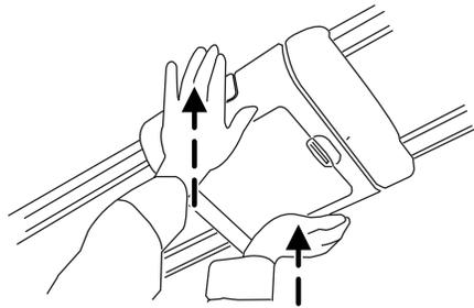
While pushing upwards with palms, grip the side latches with fingers and squeeze.
