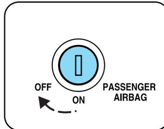
2. When the ignition is turned to the ON position the “passenger airbag off” indicator light illuminates briefly, momentarily shuts off and then turns back on. This indicates that the passenger air bag is deactivated. Refer to *Front passenger sensing system* in this chapter.
