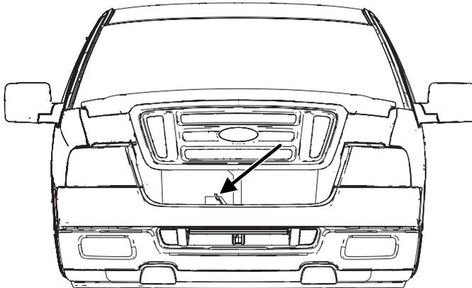
2. Go to the front of the vehicle and release the auxiliary latch that is located on the front bumper under the grill.
