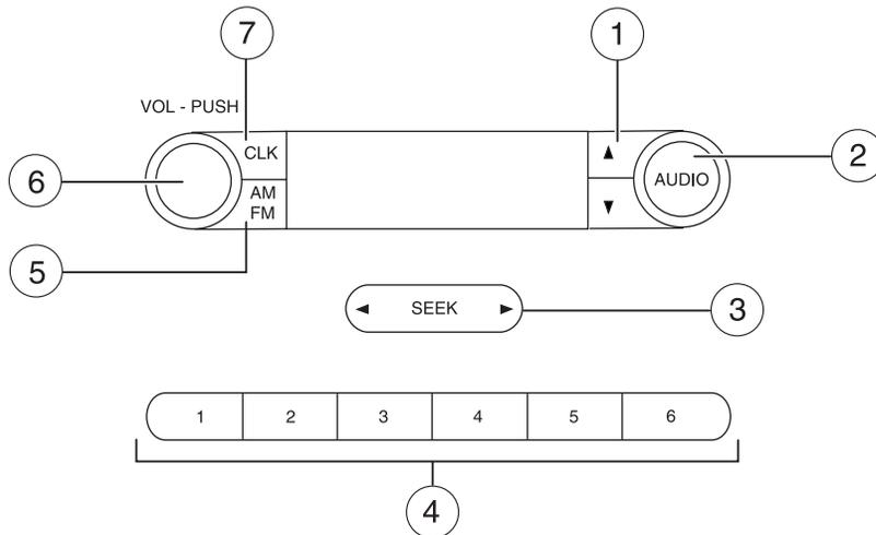
1. **▲ / ▼ Tune:** Press to manually go up or down the radio frequency. Also use in menu mode to select various settings.
