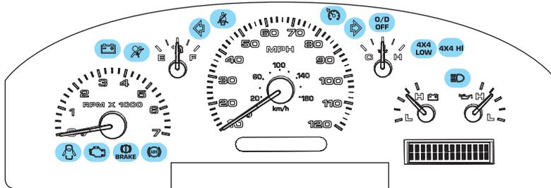
Warning lights and gauges can alert you to a vehicle condition that may become serious enough to cause expensive repairs. A warning light may illuminate when a problem exists with one of your vehicle's functions. Many lights will illuminate when you start your vehicle to make sure the bulb works. If any light remains on after starting the vehicle, have the respective system inspected immediately.
