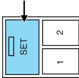
A position can only be recalled when the transmission gearshift is in Park. A memory position may be programmed at any time.
