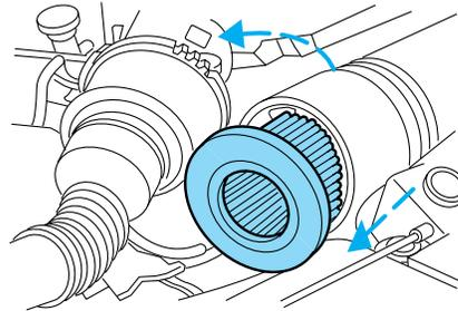
4. Install a new air filter element.
