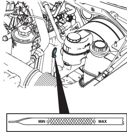
5. Locate and carefully remove the engine oil level indicator (dipstick).
