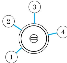
2. Turn ignition from the 3 (ON) position back to the 1 (OFF/LOCK) position in order to remove the first **coded key** from the ignition.
