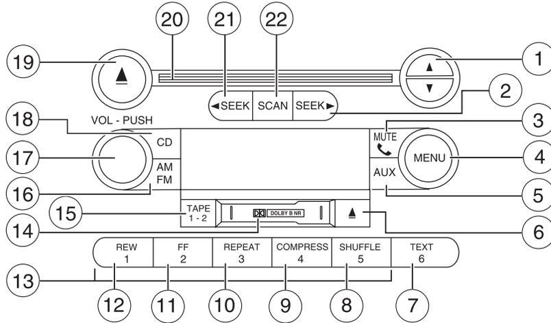
1. **▲ / ▼ Tune:** Press to manually go up or down the radio frequency. Also use in menu mode to select various settings.
