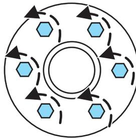
7. Position the jack according to the following guides and turn the jack handle clockwise until the wheel is completely off the ground.
