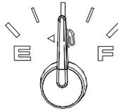
The arrow next to the fuel pump icon indicates which side of the vehicle the fuel filler door is located.
